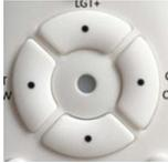
to control the brightness [dimming] (up/down buttons) and to control the colour temperature from 3000K Warm White through to 6000K Daylight (left/right buttons).
